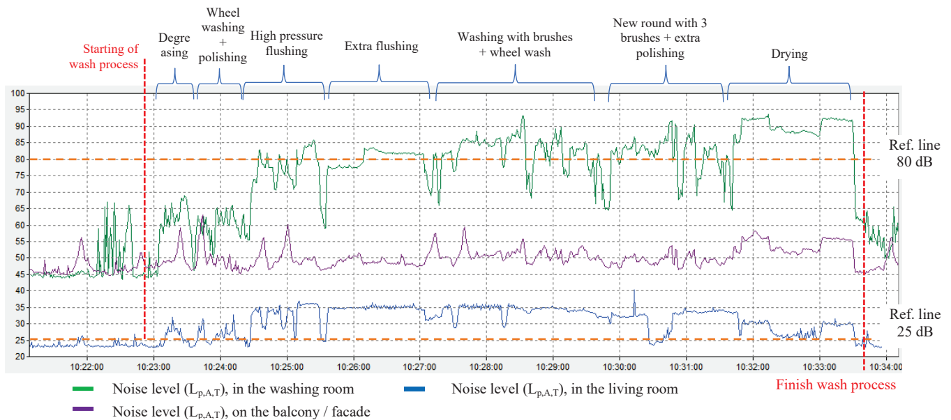
Figure 3: Noise measurements in the car wash and in the apartment, living room.
