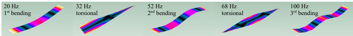
Figure 9. Natural frequencies and mode shapes for a tested 60 mm CLT panel made of spruce, length 4.0 m.
