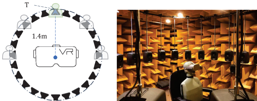
Figure 2 – Sketch of the recreation system. (Left: top view of the loudspeaker array of 24 loudspeakers in a circle of 1.4m radius, the VR position indicates the seat for the participants, the shaded portrait indicates the relative positions of the recorded avatar and actors reflected in the loudspeaker array; Right: an illustration of a test participant during the test, an audio cable was connected to the VR headset, which sent timestamp to Reaper for synchronization.)
