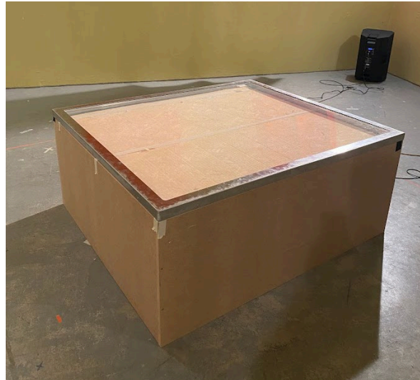
Figure 2. Basic experimental setup in the reverberation chamber (A): a 61 cm high wooden box filled with 60cm of mineral wool is used to absorb the acoustic energy that is transmitted through the membrane.
