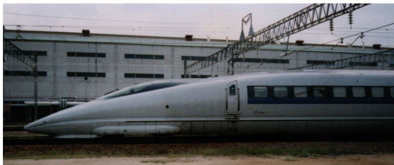
Figure 10: Optimum nose shape of series 500 Shinkansen train (JR West).
