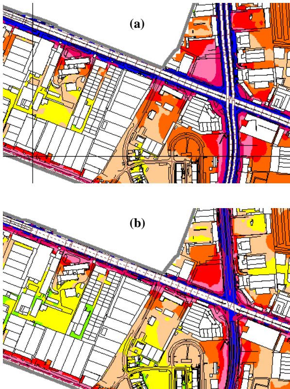
Figure 3 - Extracts of noise maps of an urban area, (a) before (b) after actions for noise reduction
