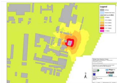
Figure 3. Strategic Noise map of the IPPC facility in Budapest XI district ( L_{DEN} )
